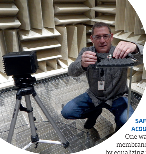
Left: Acoustic testing inside Gore's anechoic chamber
